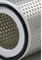
EMW<sup>®</sup> cartridge filters are available in ISO 16890 (formerly EN 779) Filter Classes and EN 1822 Filter Classes E10-H14. Their minipleat filter medium is securely mounted on the plastic frame with a cast airtight joint. A continuous foamed-in-place seal over the joint further ensures airtightness. A perforated metal guard is available as an option for additional stability under high aerodynamic stress.
